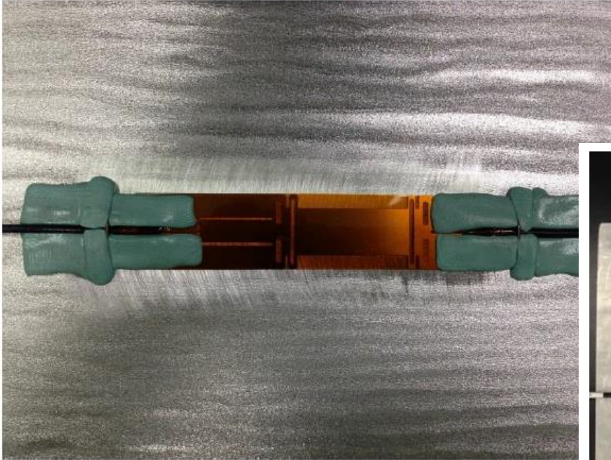
Surface Prep Area
